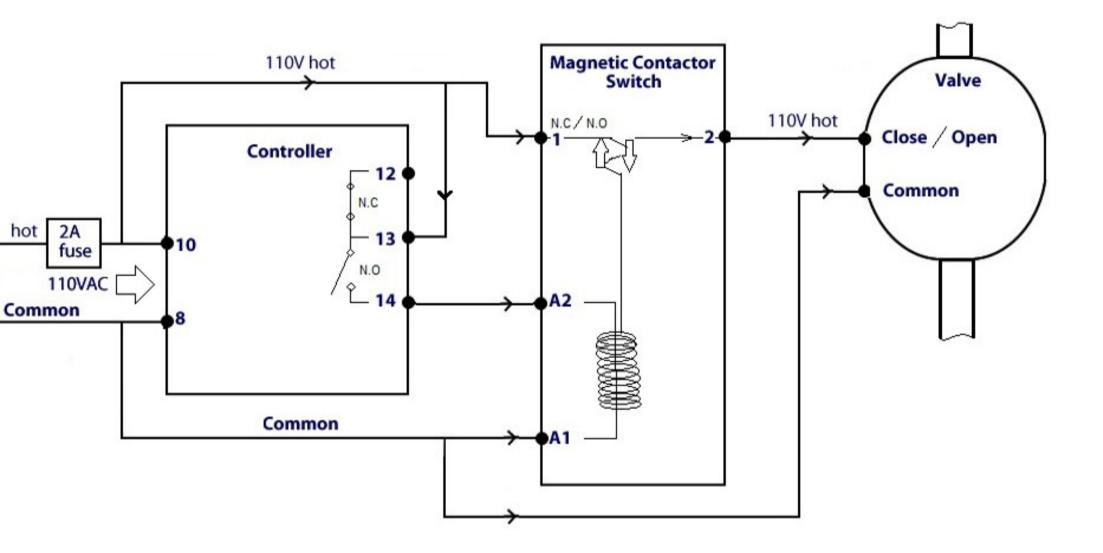
Notes: 1) The schematic above is an example. In this example, the valve will open when the TDS level hits or exceeds the set point.
