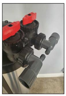
11. Connect the first tank in sequence to the second by running a line from the "Up Flow" inlet of the first tank to the "Down Flow" inlet of the second tank.
