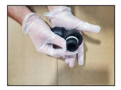
11. Lubricate the O-rings on the supplied bypass with the silicone grease. Install the bypass on the tank and fully tighten the retaining nuts. The bypass will move slightly once tight. It is made to flex and move and will not be rigid. Be sure the O-rings are lubricated on the elbow connectors previously assembled. Install the elbows in the bypass valve and tighten the retaining nuts. These will move when tight. They are made to flex just like the bypass valve connections.
