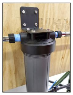
18. Place a bucket under the outlet port (downflow inlet) of the Bodyguard Whole House Chemical Removal Filter tank or run a line from the outlet port of the tank to a drain. Place the bypass in the service position.
