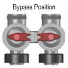
NOTE: If you see any actual pieces of bone char, immediately bypass the system. If pieces of bone char are coming out of the fluoride tank, there could be an internal problem. Small fines or tinted water is normal.
