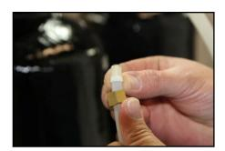
8. Push the brine line in the control valve until it stops. Then push the nut down on the fitting and tighten it hand tight. Use an adjustable wrench to tighten the nut an additional 1/2 turn.
