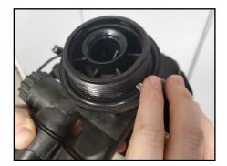
7. Install the upper basket on the bottom of the valve by lining up the tabs then turning the basket clockwise to lock it in place. Place the upper basket over the distributor tube and push the valve onto the tank. Thread the valve on the tank by turning it clockwise. Be sure not to cross thread the valve on the tank.
