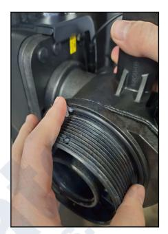
8. Align the distributor tube with the center port on the bottom of the valve and push the valve onto it and the tank. Thread the valve on the tank by turning it clockwise. Be sure not to cross thread the valve on the tank. Repeat this process for each valve in the system.
